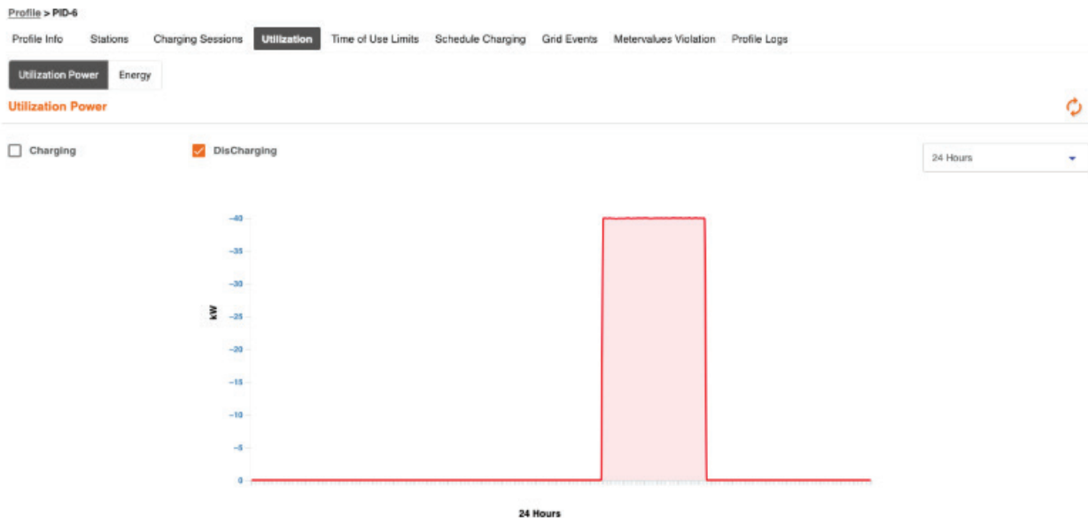
Figure 7: Representative four-hour discharge event at 40 kW for a bidirectional charger deployed at Lynch Bus Lines (Source: EVGateway)
